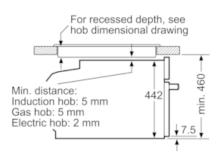
measurements in mm
